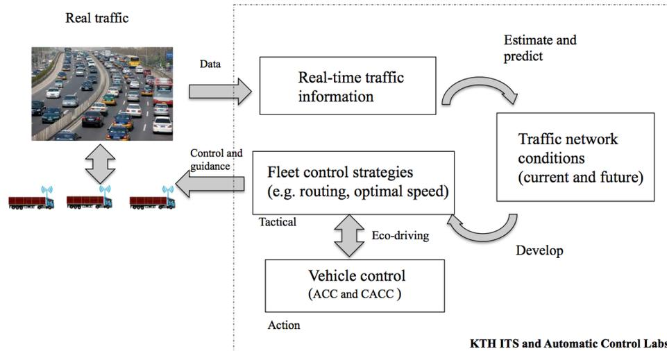
Figure 1. The concept framework of an intelligent fleet management system based on dynamic vehicle sensing and communications.
